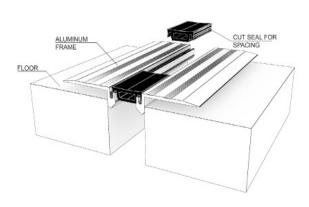
Install the architectural joint system on a level surface within the blockout. To determine blockout depth, deduct thickness of floor finish from frame height
