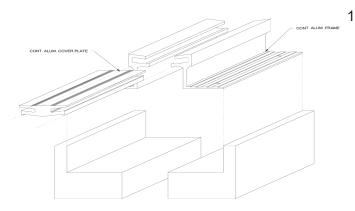
Install the architectural joint system on a level surface within the blockout. To determine blockout depth, deduct thickness of floor finish from frame height. Make sure top of frame is level with the finished floor height. This may require adding leveling compound to raise the tops of the frames
