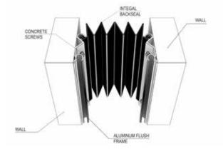
4. Trim excess length of the backseal at the base of the wall
