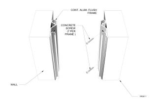
3. Measure the wall height and making it slightly longer than required. Install seal in one continuous piece. Starting at the top of the joint, insert the seal lugs into the frame receptacles
