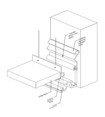
7. Press the Santoprene seal into the recessed slots of the frames until the seal is flush with the bottoms of the frames
