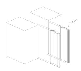
1. Install the architectural joint system frame against the adjacent wall. Transfer the location of the bottom edge of the recessed frame to the wall using a marker
