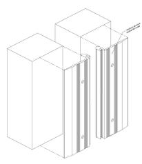
Install the architectural joint system frame against the adjacent wall. Transfer the location of the bottom edge of the recessed frame to the wall using a marker
