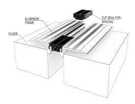
Install the architectural joint system on a level surface. This may require adding leveling compound to raise the tops of the frames
