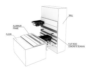
7. Press the Santoprene seal into the recessed slots of the frames until the seal is flush with the bottoms of the frames
