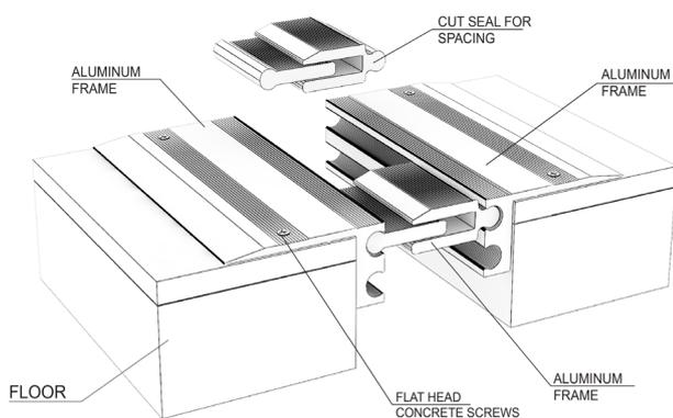
1. Install the architectural joint system on a level surface within the blockout. To determine blockout depth, deduct thickness of floor finish from frame height. Make sure top of frame is level with the finished floor height. This may require adding leveling compound to raise the tops of the frames
